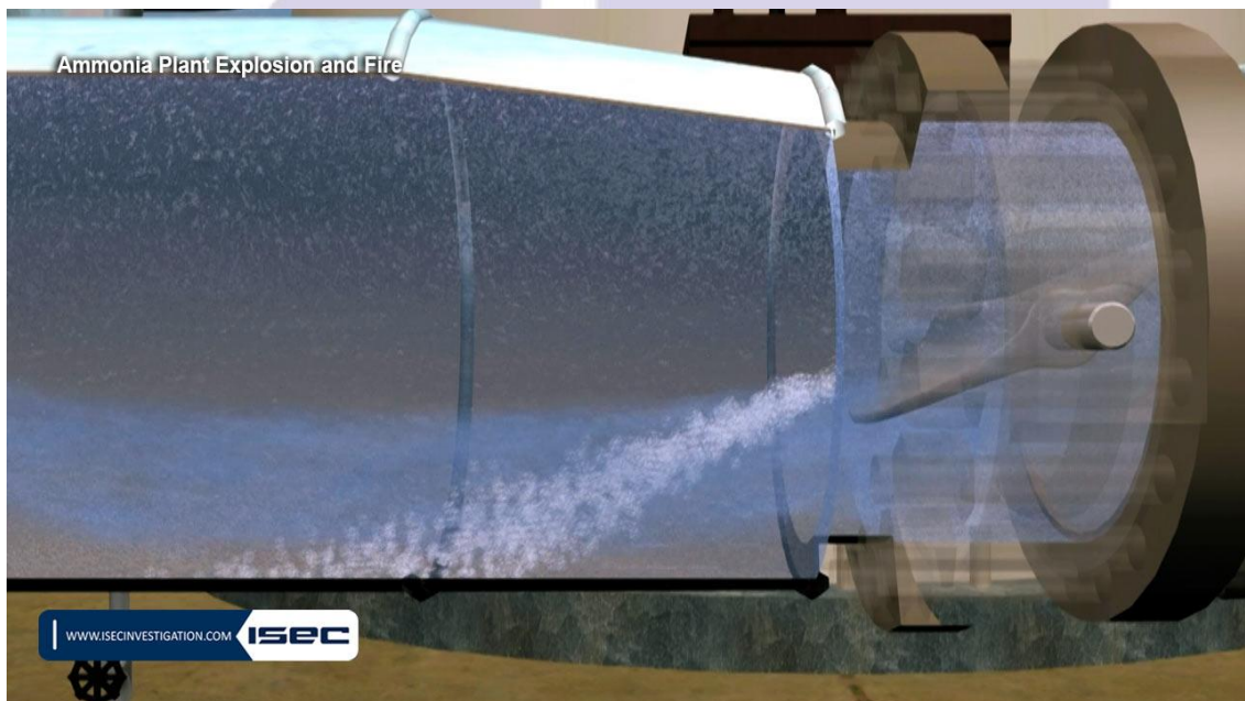
Figure 3. The FV-2004 control valve adjusted on 60%
