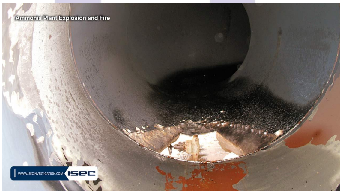
Figure 2. Corrosion factor of wet CO 2
