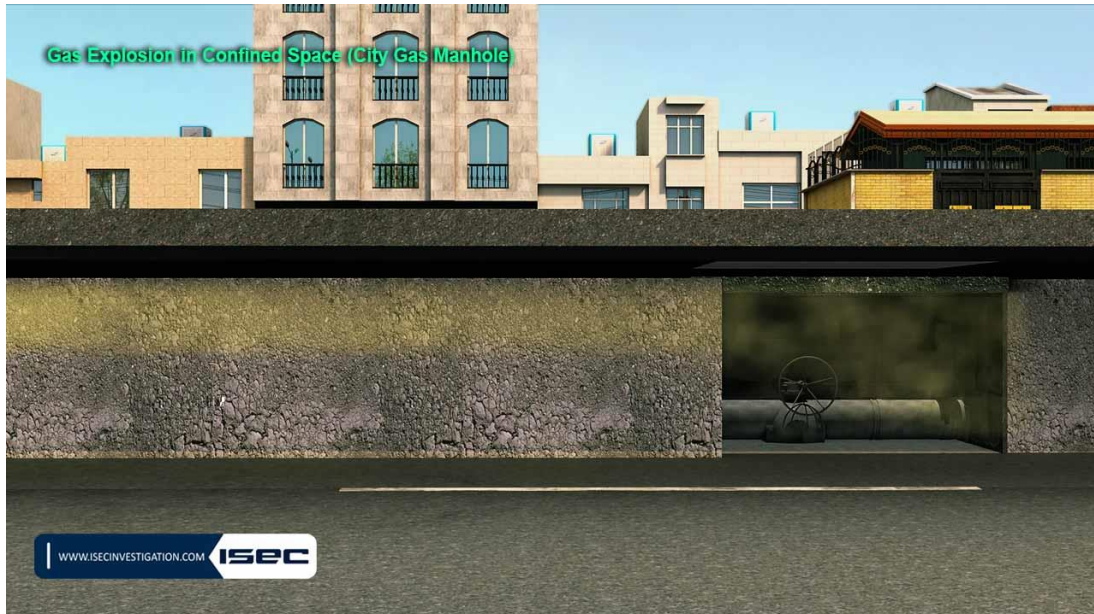
Figure 1. The gas leak entered the gas manhole from under the asphalt layer
