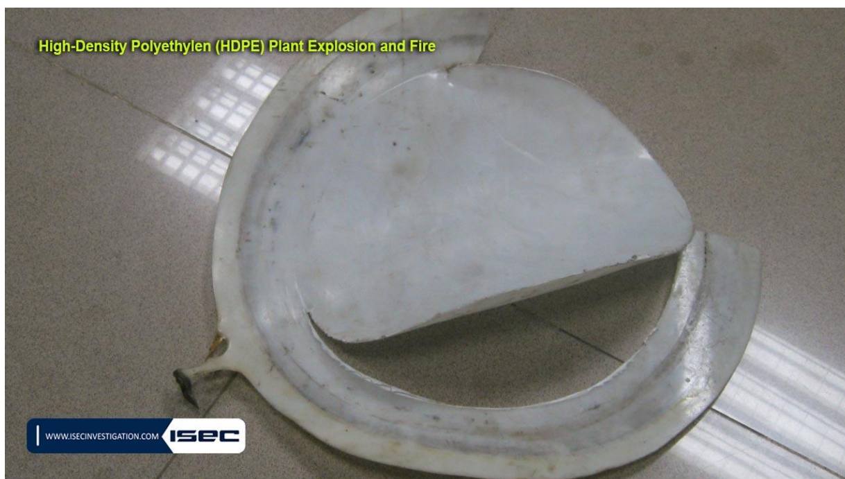
Figure 1. Teflon spade flange instead of steel type
